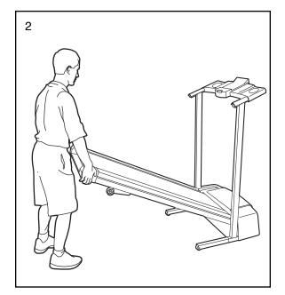
Hold the Right Handrail (94) at an angle as shown and insert the upper end into the Right Upright (11). Keep the lower end of the Handrail away from the treadmill to avoid scratching the finish. Next, rotate the lower end of the Handrail to the position shown by the dotted line.
